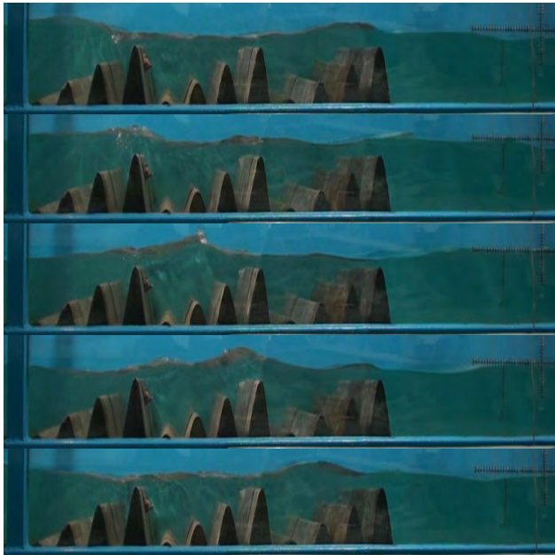
Fig. 5 Attenuation process of incident wave by combinations of three sets of rapidly varied sinusoidal breakwater at T = 1.0 s when w/h = 0.4
