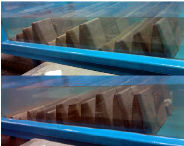
Fig.3 Illustration of composite sinusoidal submerged breakwaters
