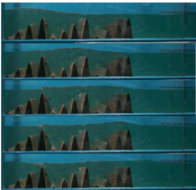
Fig. 6 Attenuation process of incident wave by combinations of three sets of rapidly varied sinusoidal breakwater at T = 1.5 s when w/h = 0.4
